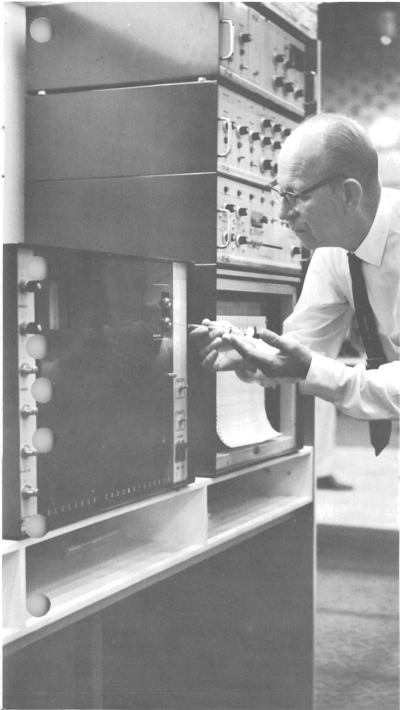
Ray Pinker, widely recognized expert in scientific crime detection, shows how a blood sample is injected into gas chromatograph for accurate analysis.
